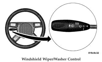
Rotate the end of the multifunction lever to the first detent past the intermittent settings for low speed wiper operation, or to the second detent past the intermittent settings for high speed wiper operation.
